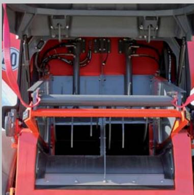
**Option: fully automatic EMC metering system**
