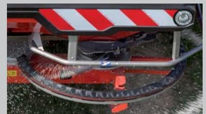
**AXMAT duo:** Radar-supported, automatic spreading pattern control
