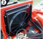
② A 21 kW oversized air-cooled radiator with double heat exchanger as standard for constant power. All hydraulic components are protected against temperature peaks.
