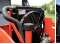
**@ A 12 kW air-cooled radiator** as standard for constant power. All hydraulic components are protected against temperature peaks.
