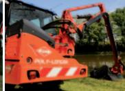
**3** Full enclosure. Over and above aesthetic aspects, the frame on the POLY-LONGER range is fully encased to guarantee full machine component protection. The frame has four storage stands and incorporates a bumper with integrated lights.
